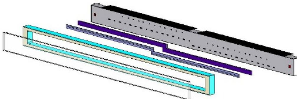
**Fig. 1.** BTDI Detector BAE Systems CCD21122 Assembly
