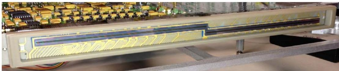
**Fig. 4.** Front view of BAE Systems CCD21122 mounted on Test Frame
