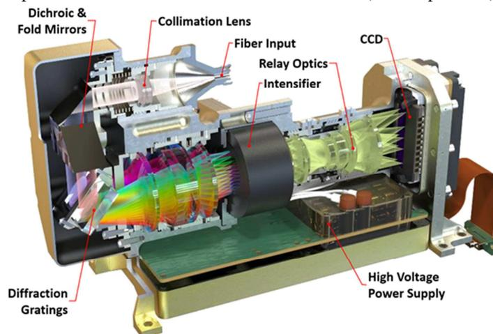
Figure 9: Transmission spectrometer design
