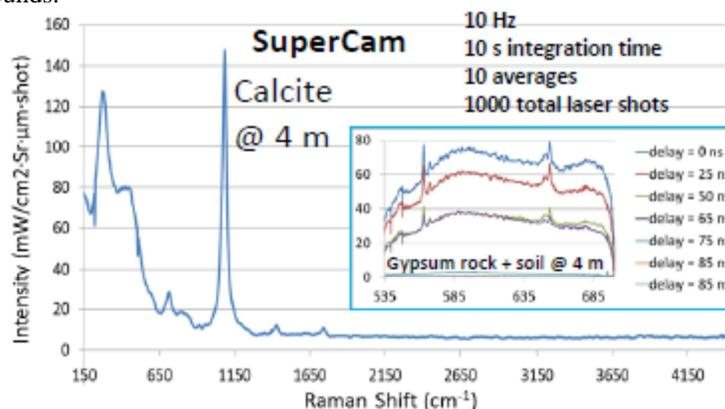
Figure 4: Raman and time-resolved fluorescence spectrum (low resolution example)
