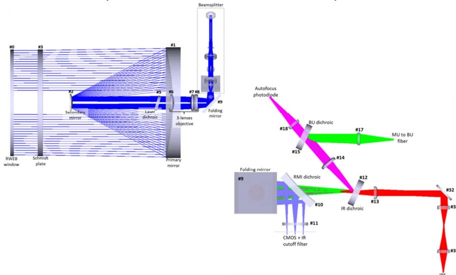
Figure 8: VIS – The collect path (left: telescope and right: beamsplitter)
