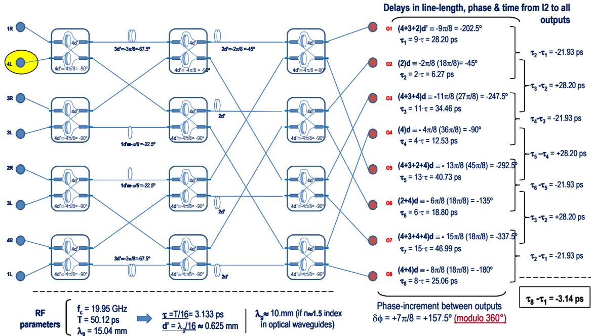
**Fig. 2.** Scheme of an optical Butler matrix of 8x8 ports implemented by optical splitters/combiners and optical delays. The squares indicate the structures working as 90° RF Hybrid. In the bottom of the figure some calculations for the matrix parameters are included. The right side includes the calculated delay and corresponding phase of the output signal when entering in the port 4L (in yellow), which corresponds with a differential phase of 157.5° between adjacent ports.
