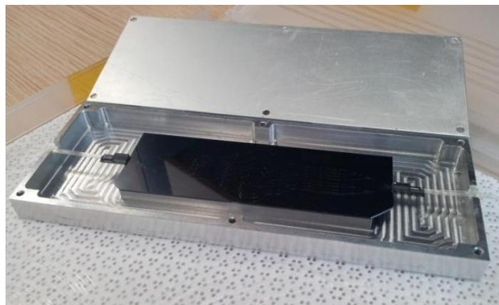
**Fig. 5.** Picture of the optical Butler matrix chip after packaging
