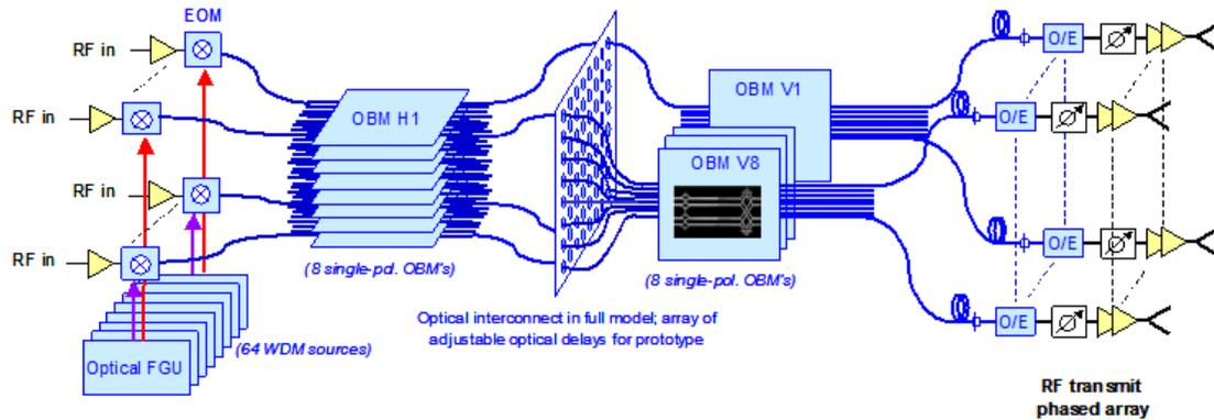
**Fig. 3.** Schematic of the baseline architecture of a transmit Optical Beamformer Network (OBN), that features the full-scale optical beam-former, the E/O and O/E conversion interfaces and all the associated optical links
