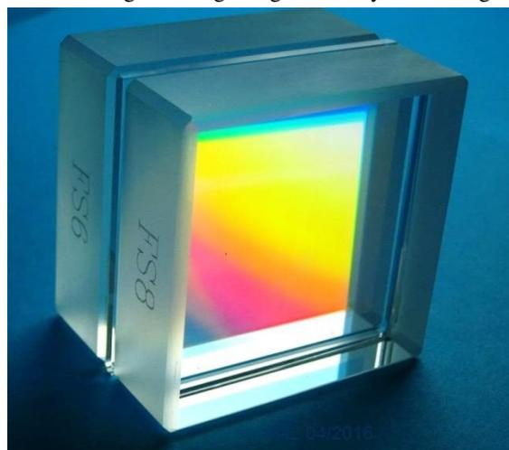
**Fig. 6.** Prism-grating-prism type bond using prism dummies of plane-parallel shape
