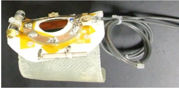
Figure 3. ^{19}\text{F} single-tuned quadrature RF coil with T/R switch in Fig. 1(a) for rabbit eye ^{19}\text{F} MR spectroscopy, consisting of a circular and 8-shaped coils to orient the magnetic field orthogonal to each other. The coil is positioned within a volume Tx/Rx coil. ^1\text{H} coil was actively detuned during the ^{19}\text{F} imaging by PIN diodes.
