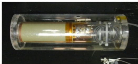
Figure 1. (a) Quadrature T/R switch, including preamplifier and (b) two single tuned quadrature RF coils for mouse imaging. A PIN diode is used to switch between Tx and Rx in T/R switch. T/R switch is capable to accept a proton-only or ^{19}\text{F}/^1\text{H} dualtune RF coil.
