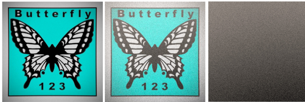
Fig. 4 The result of the simultaneous calculation of the image illuminance for three different criteria. From left to right: main image, main image and stray illumination caused by light scattering on the aperture, and stray illumination caused by light scattering on the aperture.
