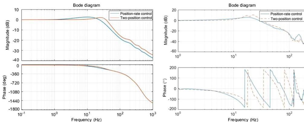
**Fig. 6** Tracking control closed-loop responses of the tip-tilt mirror system: (a) simulation and (b) experiment.
