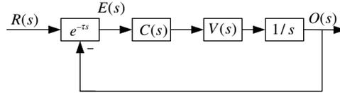
Fig. 4 Functional block diagrams of the time delay control system with position-rate control.
