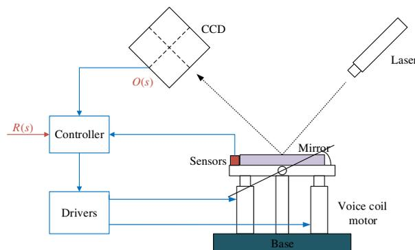
**Fig. 1** Configuration of an image-based tracking control system for tip-tilt mirror.
