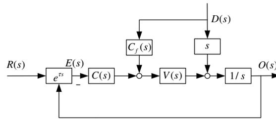
Fig. 10 Functional block diagrams with disturbance feedforward control.
