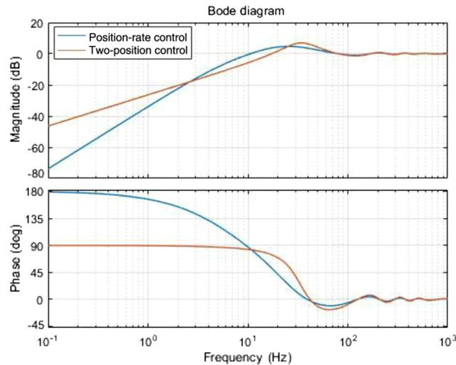
Fig. 7 Bode responses of two error transfer functions.
