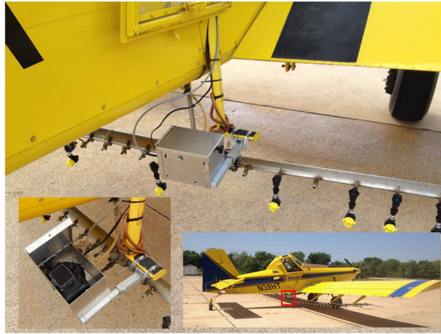
Fig. 2 A Nikon camera mounted on the right step of an Air Tractor AT-402B. A GPS receiver and a video monitor integrated with the camera are mounted in the cockpit.
