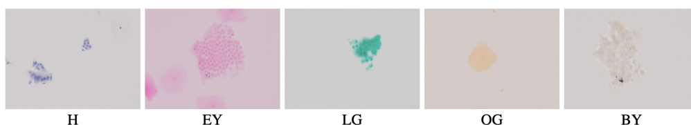
Fig. 2 Examples of single-stain images used to calculate the spectral absorption coefficient matrix \mathbf{H} .
