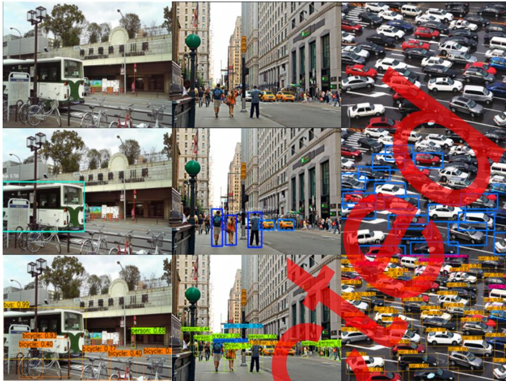
**Fig. 5** Object detection results of a single picture: (a) few object image, (b) medium object image, (c) dense object image, (d) few object image (YOLOv2), (e) medium object image (YOLOv2), (f) dense object image (YOLOv2), (g) few object image (YOLOv3), (h) medium object image (YOLOv3), (i) dense object image (YOLOv3).
