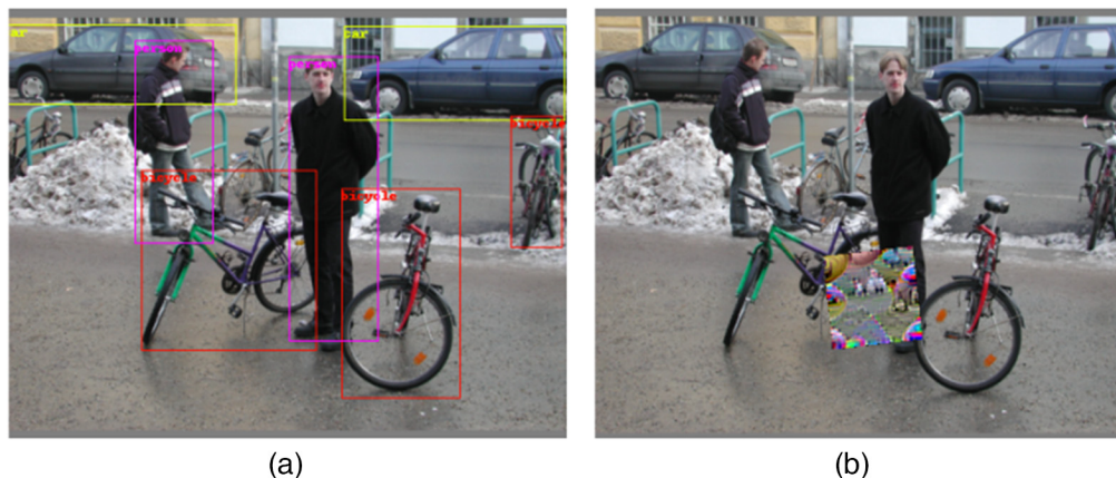
Fig. 2 Example of our patch on the Inria test set, which is not only effective for pedestrians but also inhibits the detection of all objects in the image. (a) Original image and (b) attack.
