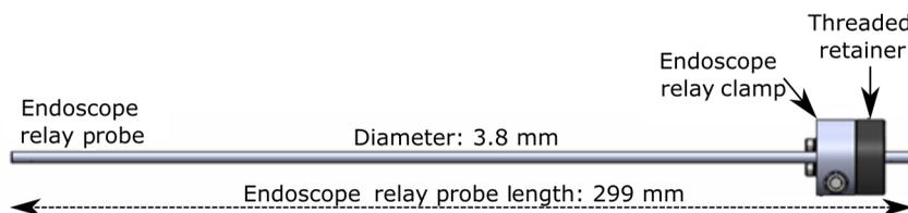
**Fig. 2** SolidWorks rendering of the endoscope assembly indicating the endoscope probe, fabricated clamp, and threaded retainer. The threaded retainer is threaded to match the 30 mm cage mounted components. This allows for quick connection to the handle section.
