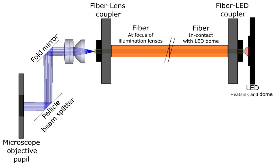
**Fig. 6** Illumination diagram showing the LED-fiber coupling and the fiber-lens coupling setup representing the expansion of the fiber to fill the microscope objective pupil.
