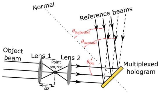
**Fig. 4** Recording geometry of the multiplexed hologram. The recording angle of the object beam,  $\theta_{\text{obj}}$ , is constant at 33.4 deg for both recordings. The reference beam angle,  $\theta_{\text{ref}}$ , changes between 34.92 deg and 31.88 deg for the surface and depth, respectively.
