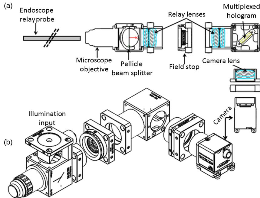
**Fig. 5** SolidWorks rendering of handle component layout. (a) Top-down view demonstrating the layout of the lenses, hologram, and camera; (b) an isometric view indicating the location of the illumination path through the pellicle beam splitter cube.
