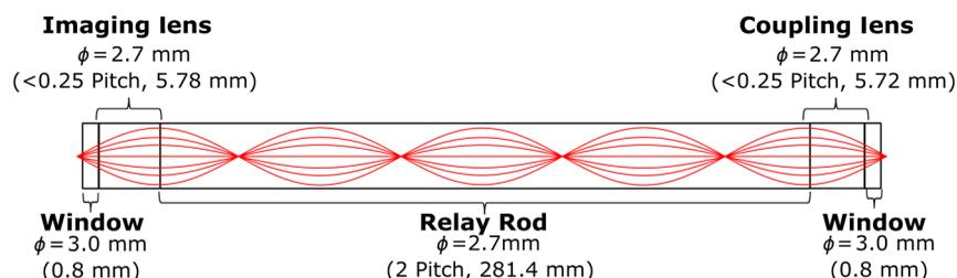
**Fig. 1** Schematic of the endoscopic probe composed of GRIN lenses. Grin components have diameters of 2.7 mm, and the windows have a diameter of 3.0 mm. The theoretical optical path from an object placed in contact with the imaging lens, being relayed through the GRIN rod, and exiting to form an image outside the window on the coupling lens side is shown.
