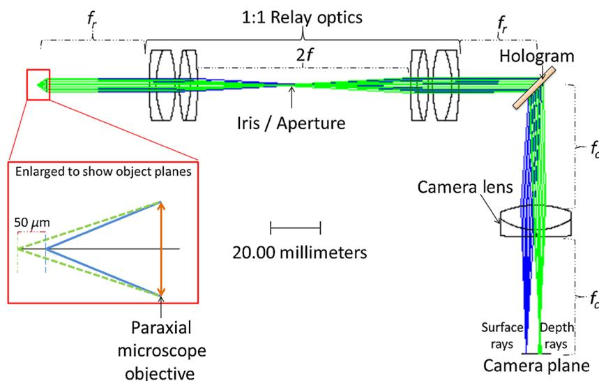
**Fig. 3** ZEMAX schematic of the handle layout. The surface (solid blue) and depth (dashed green) images in the inset are shown to originate from on-axis positions in the object and are then displaced by the holographic element to fill two regions on the camera as indicated by text in at the camera plane. Spacing of the lens elements are provided in the dashed brackets.
