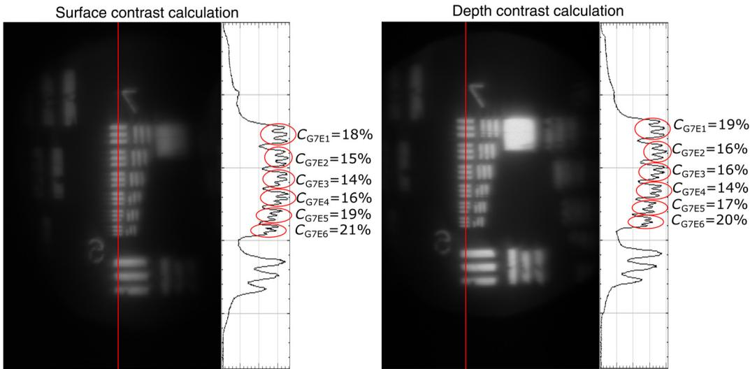
**Fig. 8** Contrast calculations for the group 7 elements in the USAF resolution chart. The lowest contrast content seen in the chart is at 14%.
