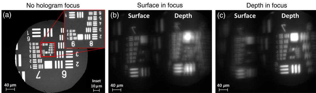
**Fig. 7** (a) Resolution test of handle components prior to addition of volume hologram and endoscope probe relay. The smallest target available on the chart is group 9, element 3 with a size of  $1.55 \mu\text{m}/\text{lp}$  ( $645.08 \text{ lp}/\text{mm}$ ). (b) Surface channel focus, (c) depth channel ( $\Delta = 50 \mu\text{m}$ ) focus [both (b) and (c) show  $4.4 \mu\text{m}$  or better resolution with the hologram and endoscope probe added].
