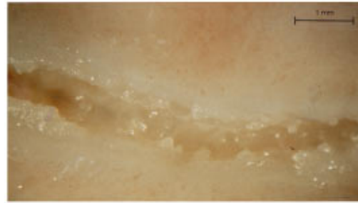
Fig. 7 Microscopic photograph of an in vitro holmium laser incision achieved in the pulse-compressed mode. Fiber, 200 \mu\text{m} ; average laser power, 2 W; prf, 10 Hz; cutting speed, 0.25 mm/s. The incision is very irregular. The incision width varies between 300 and 800 \mu\text{m} .
