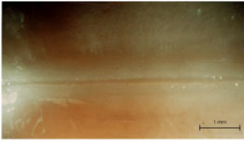
Fig. 5 Microscopic photograph of an in vitro holmium laser incision achieved in the free-running mode. Fiber, 200 \mu\text{m} ; average laser power, 2 W; prf, 10 Hz; cutting speed, 0.25 mm/s. The histology shown represents the upper limit of channel dimensions with these parameters.
