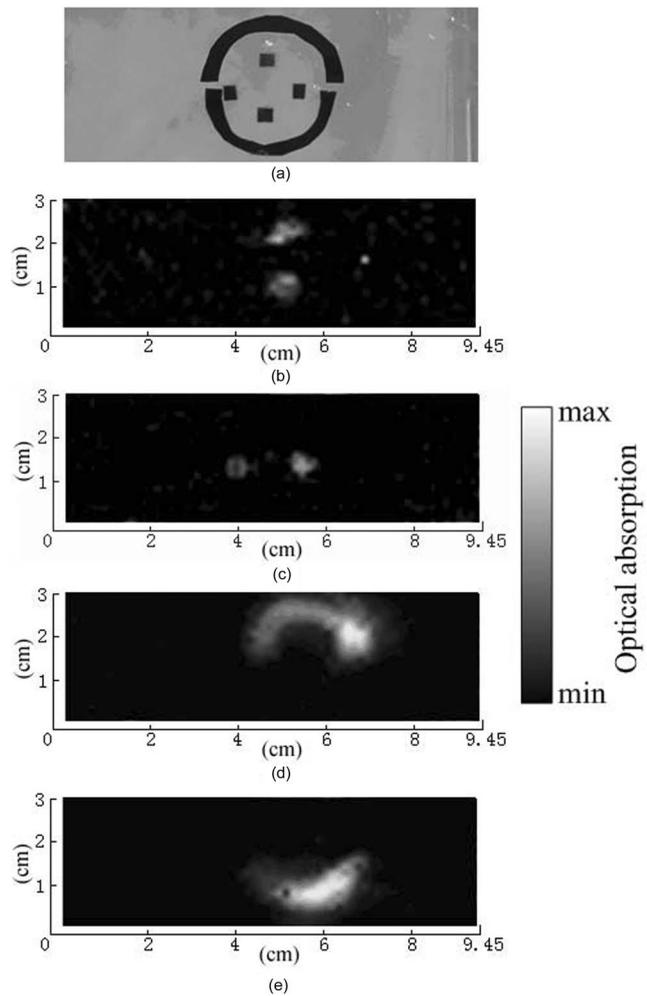
Fig. 3 Front elevation of (a) the sample, which consists of four different patterns: two lengthways black adhesive tape dots stuck to the front, two transverse black adhesive tape dots stuck to the second layer, a lower half ring of black adhesive tape stuck to the third layer, and an upper half ring of black adhesive tape stuck to the back of three pieces of polymethylmethacrylate. (b-e) are the corresponding reconstructed PA images of the four parts of the sample.
