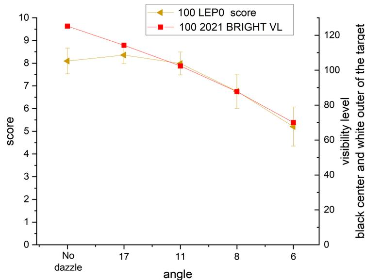
**Fig. 10** Estimated marginal means of scores for the standard ballistic goggles (LEP0) and 100% contrast target (left scale) compared to the estimated VL for the inner black center of the target with the white outer rings in the corresponding conditions. Error bars for the scores stand for 95% confidence intervals.
