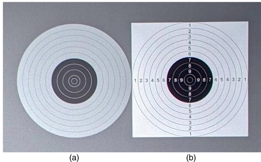
**Fig. 2** Photo of (a) the 25% contrast target and (b) the 100% contrast target. The 0.5% contrast target (not shown) had the same shape as the 25% contrast target.
