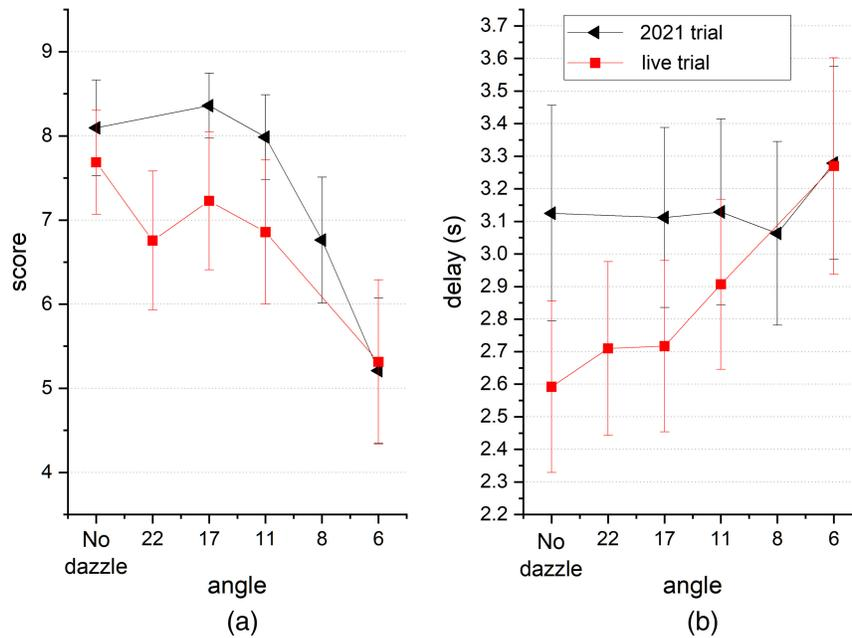
**Fig. 9** Estimated marginal mean shooting (a) scores and (b) delays for the 100% contrast target and standard ballistic goggles, obtained from the 2021 shooting simulator trial (shown in black), as well as the estimated marginal means from the live shooting trial<sup>13</sup> (shown in red). The error bars stand for 95% confidence intervals.
