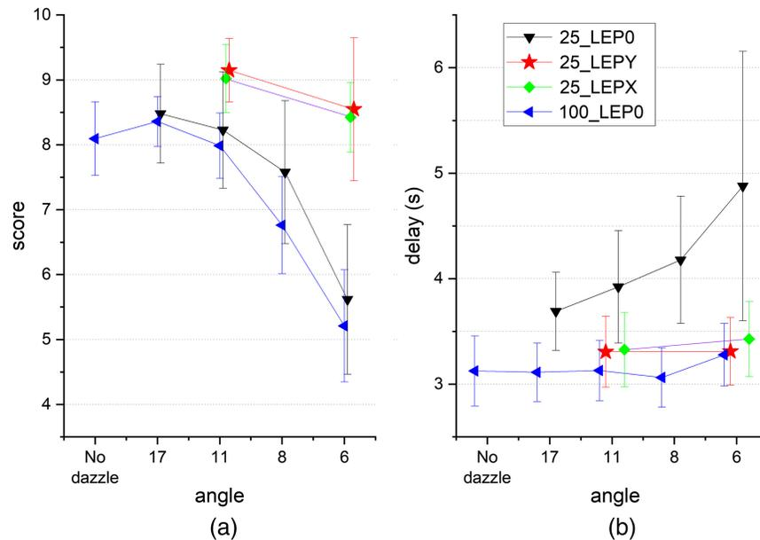
**Fig. 3** Subset of the estimated marginal means of (a) scores and (b) delays from the 2021 and main 2022 campaigns as estimated by the linear mixed model. Error bars stand for 95% confidence intervals. Codes shown in the legend represent the contrast of the target followed by the designation of the worn goggles. The curves are slightly offset on the x-axis for visual clarity.
