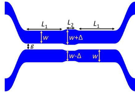
Fig. 2 Schematic of a broadband asymmetric DC (not to scale).
