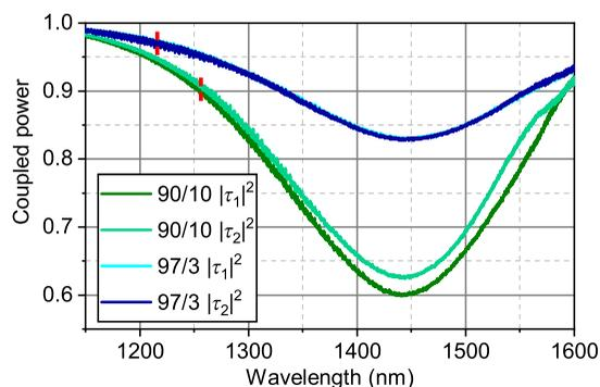
**Fig. 4** Measured through-coupling spectra of the 90/10 and 97/3 broadband DCs. The red dashed line indicates 90.5% and 97.0% coupling, respectively.
