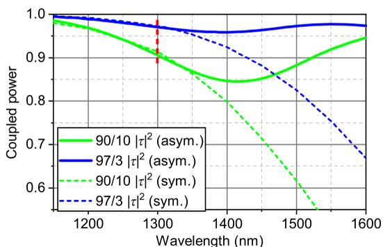
**Fig. 3** Simulated through coupling  $|\tau|^2$  for the 90/10 and 97/3 DCs. The solid lines correspond to the broadband asymmetric DC, whereas the dashed lines correspond to a symmetric DC, shown for reference (see text). The red line indicates the filter resonance wavelength of 1300 nm.
