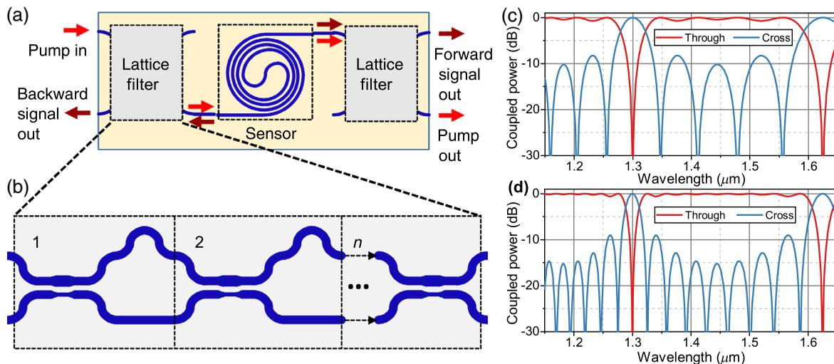
Fig. 1 (a) System design for a PIC transducer with integrated broadband filters. (b) An  $n$ -stage LF comprising  $n$  unbalanced propagation stages and  $n + 1$  broadband DCs. (c) The calculated response of a four-stage LF with optimized coupling. (d) The calculated response of an eight-stage LF with optimized coupling.
