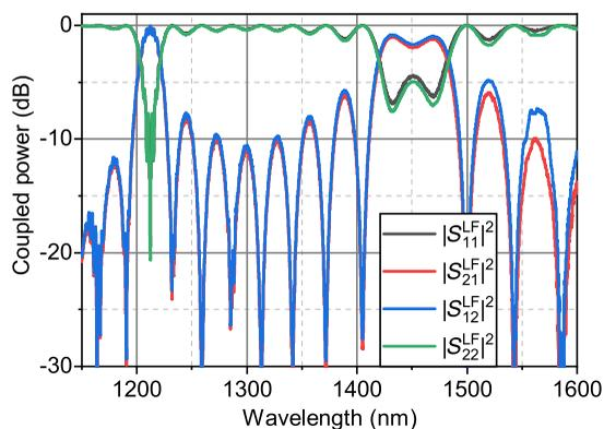
**Fig. 6** Measured through- and cross-coupling spectra of the eight-stage LF.
