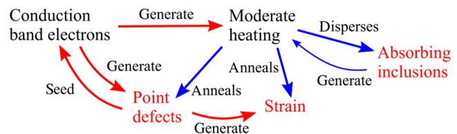
**Fig. 3** Possible modifications of pre-existing fabrication defects during the incubation pulses.
