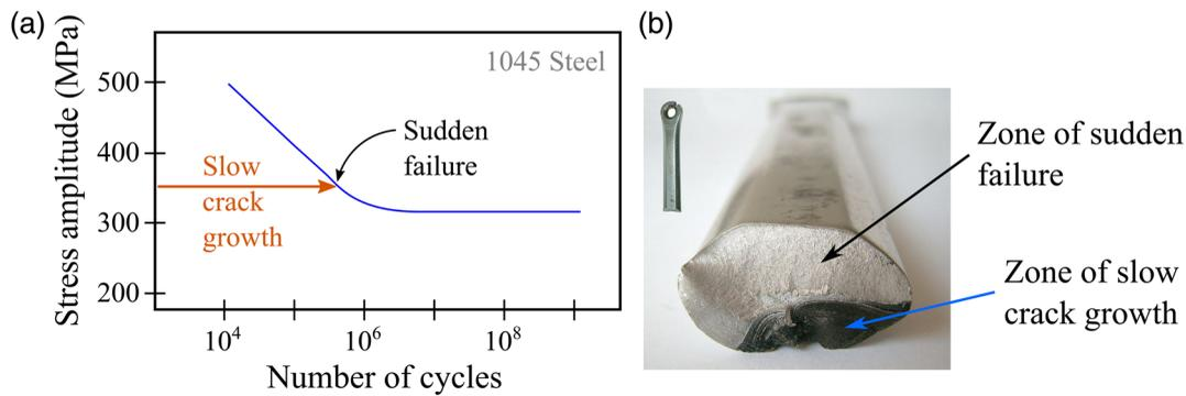
**Fig. 1** Information on mechanical fatigue damage. (a) Mechanical fatigue damage in steel, according to Ref. 12. A chosen stress amplitude is applied and removed for a high number of cycles. During the first cycles, a small crack is initiated. The crack then grows slowly until the work piece breaks suddenly. (b) Photograph of an aluminum part that was subject to fatigue failure.<sup>13</sup>
