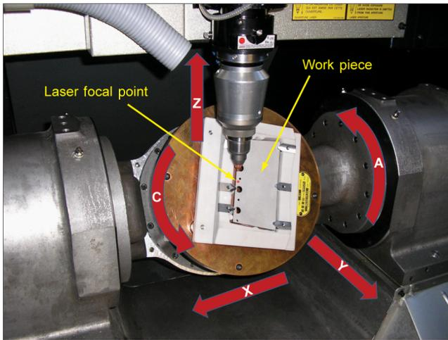
Fig. 3 Configuration of a five-axis laser drilling machine tool.
