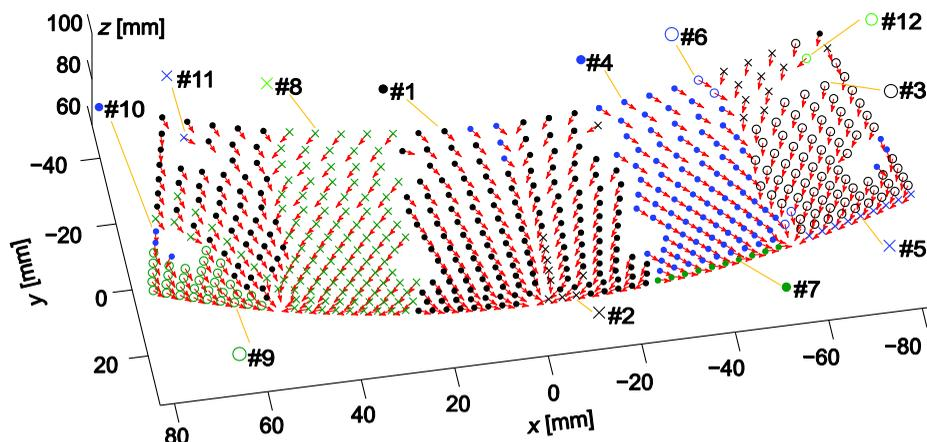
Fig. 4 Hole clusters and orientations for a turbine combustion chamber panel.
