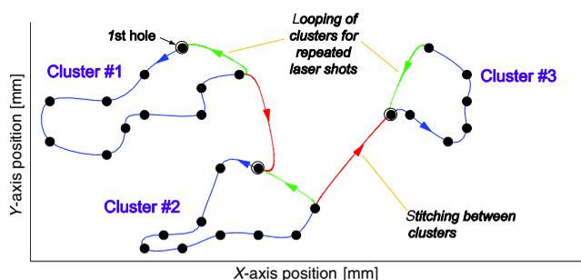
**Fig. 8** Earlier developed strategy in Ref. 1 for on-the-fly drilling trajectory generation,<sup>1,3</sup> comprising of (1) optimizing each hole cluster separately and (2) looping and stitching of individual clusters using time-optimal connections.
