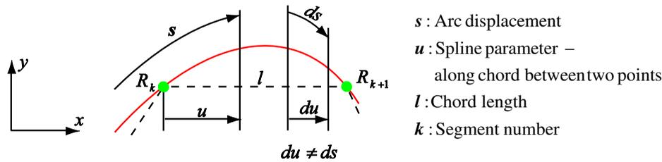
Fig. 7 Parameter ( $u$ ) and actual path ( $s$ ) increments in spline interpolation.
