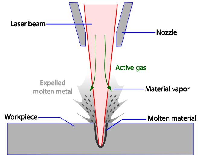
**Fig. 1** How laser drilling works: the laser melts and vaporizes the material. The vapor pressure expels the molten material from the hole.
