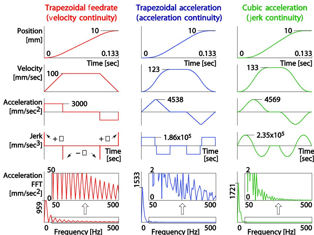
Fig. 6 Time- and frequency-domain comparison of three different trajectory types.
