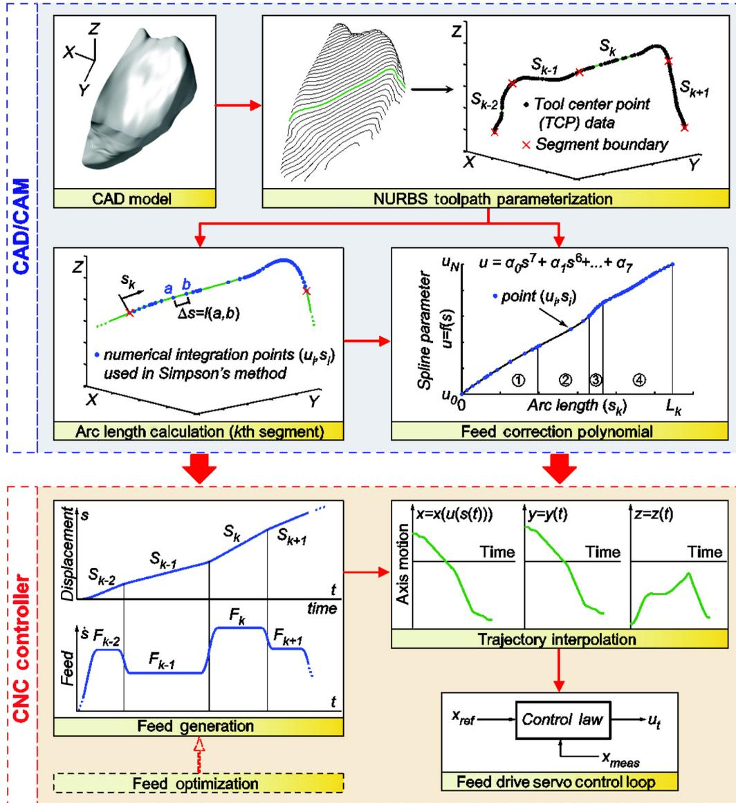
Fig. 5 Overview of trajectory generation in machine tools (From Heng<sup>25</sup>).
