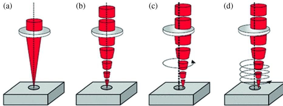
**Fig. 2** Laser drilling techniques: (a) single pulse drilling, (b) percussion drilling, (c) trepanning, and (d) helical drilling (from left to right).<sup>17</sup>
