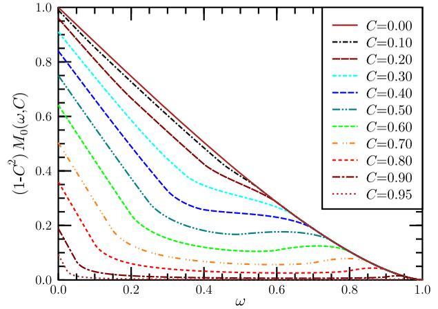
**Fig. 3** Unnormalized annular aperture system MTF curves for the  $C = D_1/D_2$  parameter ranging from 0.0 to 0.95.
