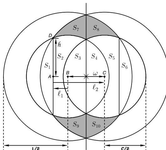
**Fig. 2** Intersection of annular apertures displaced center-to-center from one another by amount  $\omega$  of unit outer diameter and inner diameter  $C = 9/14$ . Subregions are labeled as  $S_1$  through  $S_{10}$ . Cross marks center of coordinate system (origin of  $\mathbf{v}$  vector space).
