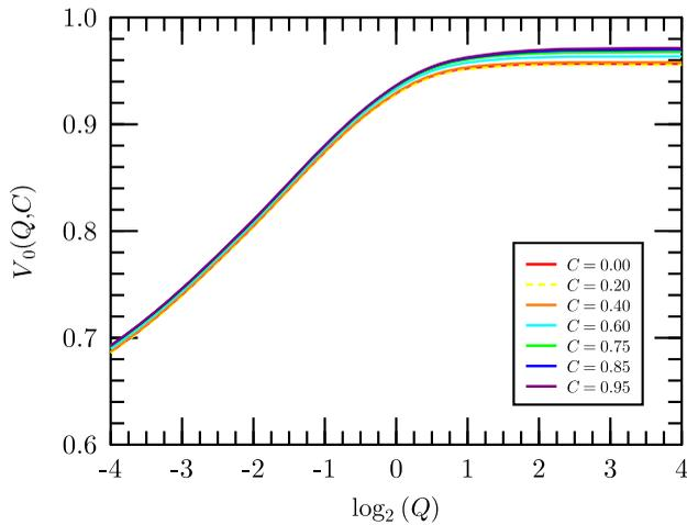
**Fig. 8** Plots of minimum  $V(\omega, X, Q, C)$  values ( $V_0$ ) as functions of increasing  $Q$  for different aperture central obscuration fractional widths  $C$ .
