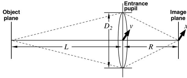
**Fig. 1** Imaging geometry of the short-exposure imaging problem where optical turbulence fluctuations exist between the object plane and the system entrance pupil.
