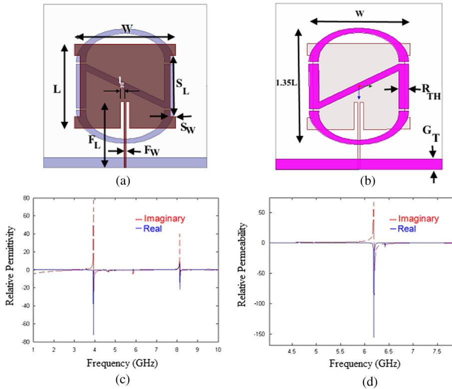
**Fig. 1** Negative refractive index inspired patch resonator. (a) Top view. (b) Bottom view. (c) Relative permittivity. (d) Relative permeability.
