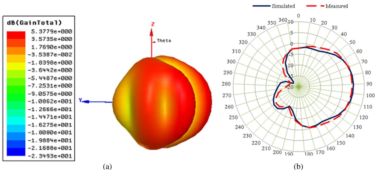
Fig. 4 Antenna radiation characteristics. (a) Polar plot. (b) Radiation pattern.
