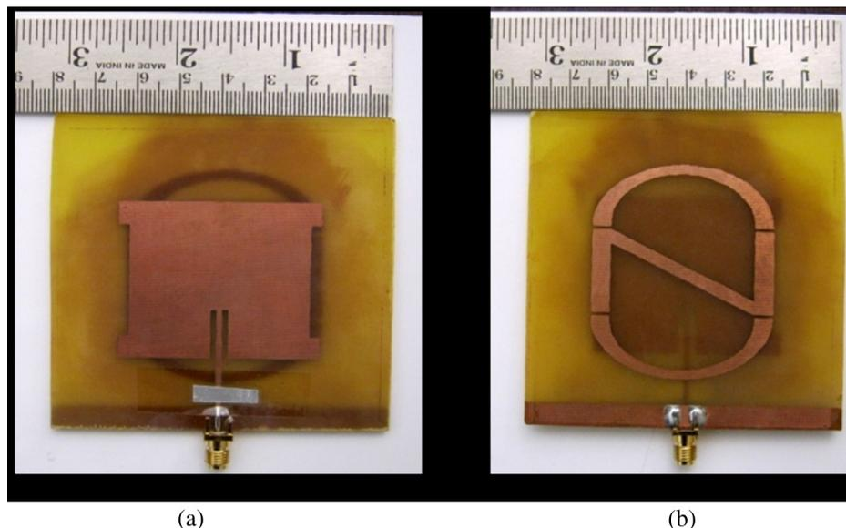
**Fig. 2** Fabricated prototype of antenna. (a) Top view. (b) Bottom view.
