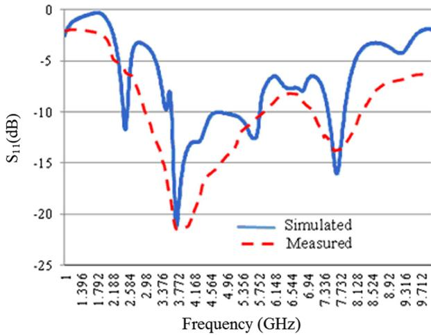
Fig. 3 Antenna return loss.
