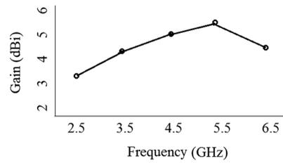
Fig. 5 Realized antenna gain.
