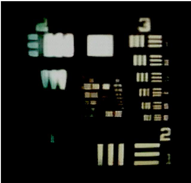
**Fig. 9** Image of AF target taken by lens 4, the half-moons.
