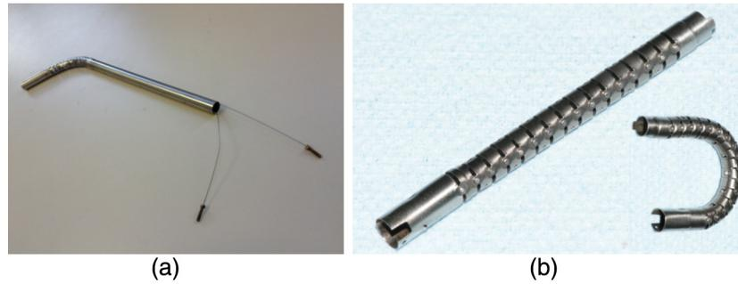
**Fig. 10** (a) Typical bending section with steering cables. Pulling the left-hand side of the cable rotates the bending section to left. (b) Close-up image of links used in bending sections employed in MARVEL (Example showed here uses 15 links to achieve  $\sim 180$  deg bend).
