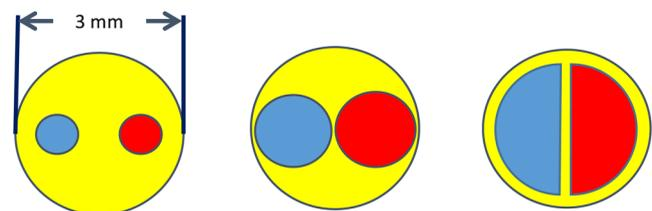
**Fig. 7** Aperture diameter and separation of bipartite filter options tested: (a) 0.6/1.2-mm, (b) osculating, and (c) half-moons.
