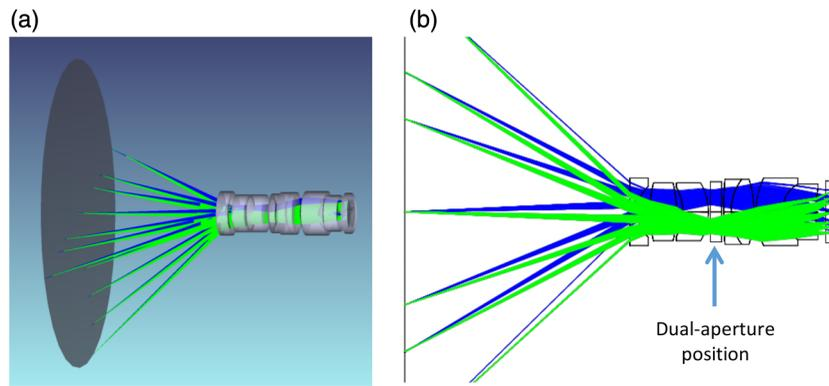
**Fig. 6** (a) Ray traces of the light passing through the lens elements. The blue and green rays represent the light path through one or the other apertures, providing left and right viewpoints. (b) The location of a dual-aperture plate. Notice that the light incident on the plate is near orthogonal.
