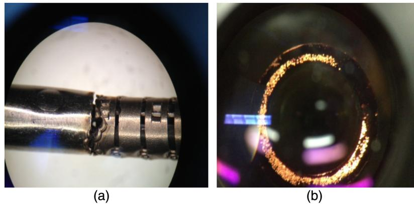
**Fig. 14** (a) Photo of the disjointed welding. (b) Photo of the illumination power lost after the joint welded for the second time due to loss of optical fibers.
