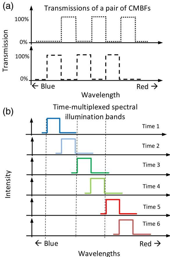
Fig. 3 Spectral schematic shows the operating principle of CMBF-based stereo imaging technique. (a) Shows transmission characteristic of the CMBF filters and (b) shows time-multiplexed SIBs synchronized to the transmission bands of the CMBF filters.
