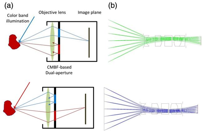
Fig. 4 Dual aperture created by a pair of CMBFs: (a) schematic drawing showing the CMBF pair opening to SIBs and (b) ray traces of the CMBF lens system simulated by an optical simulation software package.
