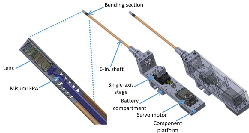
**Fig. 11** Mechanical drawing of the 3-D-MARVEL layout.
