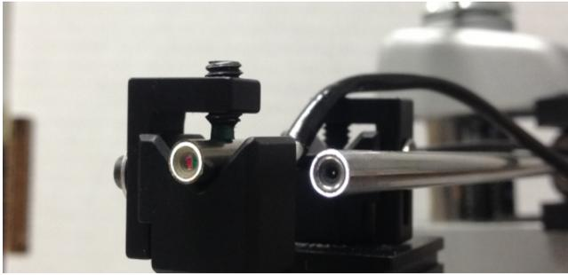
**Fig. 8** Picture of the custom 3-D endoscope (left) next to a commercial 2-D endoscope to show the dimensional comparability. Notice that in the left endoscope half moon CMBF filters can be seen.
