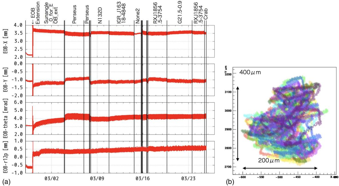
**Fig. 3** (a) The time history of the center position of the EOB (EOB-X and EOB-Y), its rotation around the spacecraft Z-axis (the launch direction) from the nominal orientation, and changes of the distance between the two corner cubes. (b) Stability of the focal plane alignment measured in about a day with CAMS after the EOB extension.
