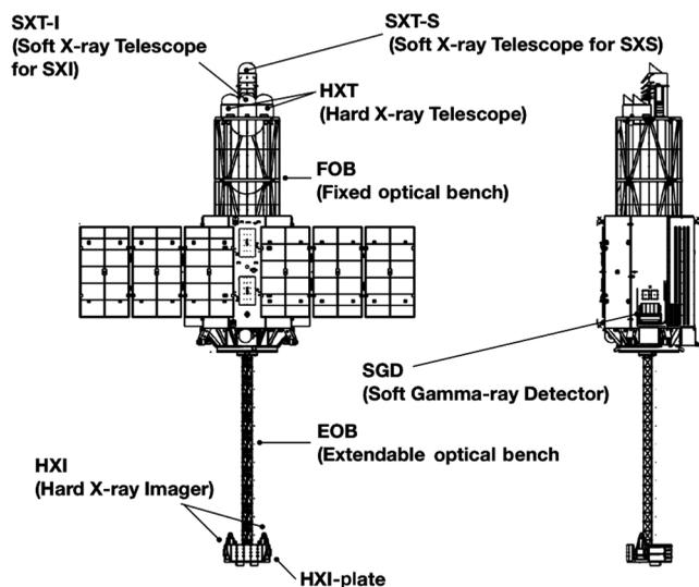
**Fig. 2** Schematic view of the Hitomi satellite with the extendible optical bench deployed. The total length of the satellite is about 14 m.<sup>8,10-12</sup> The SXS instrument is equipped in the opposite side of the solar paddle.
