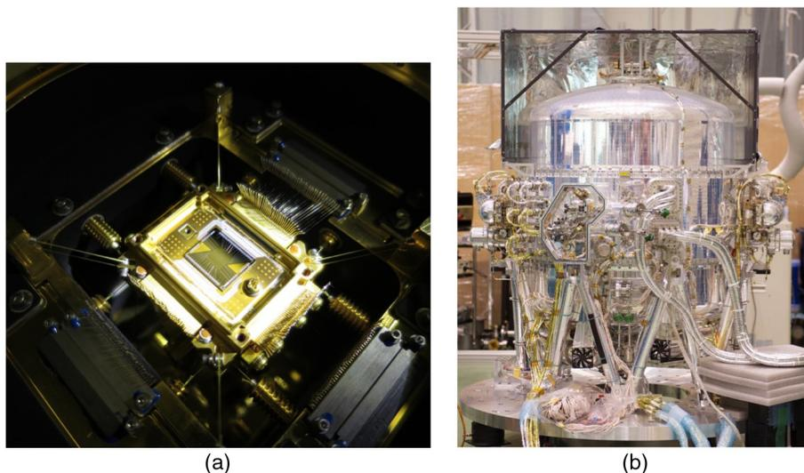
**Fig. 5** Photographs of (a) SXS sensor and (b) SXS dewar. The sensor was suspended from the outer structure using Kevlar, and electrical connections to the housing were made using tensioned wires to reduce the sensitivity to microphonics. The outer shell of the dewar is 950 mm in diameter.
