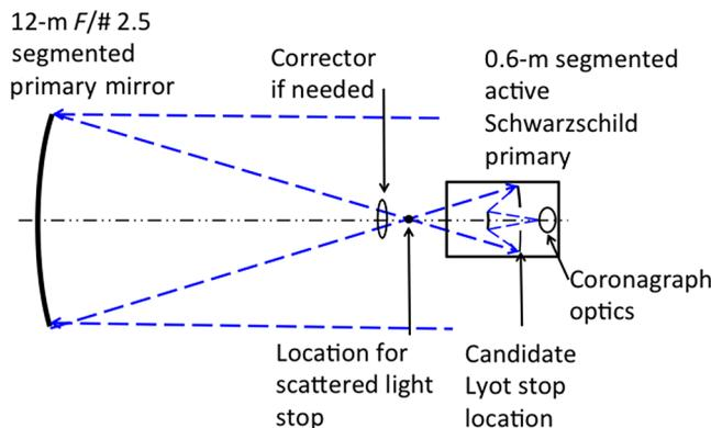
**Fig. 4** Prime-focus schematic concept for the EST system. A PFIA is shown docked at the right end of the metering structure, 30 m from the vertex of the PM that separates the primary from the PFIA. (Illustrative—not to scale.)
