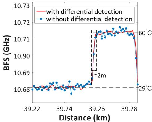
**Fig. 6** Measured BFS at the far-fiber end from 39,220 to 39,285 m (a) without and (b) with differential detection.
