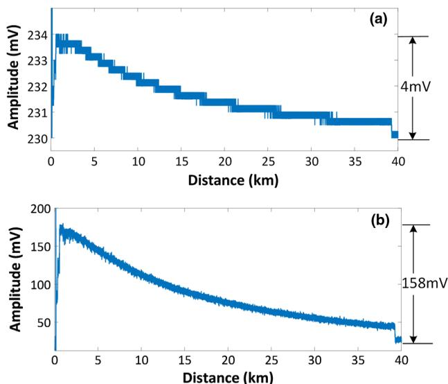
Fig. 4 Measured BOTDA time traces (a) without DC cancellation and (b) with DC cancellation along  $\sim 40$ -km sensing fiber at the sweeping frequency of 10.68 GHz.
