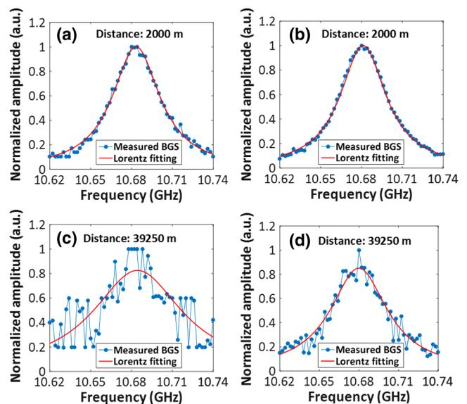
Fig. 5 Measured BGSs and their Lorentz fittings (a, c) without and (b, d) with differential amplification at the distances of 2000 and 39,250 m, respectively.
