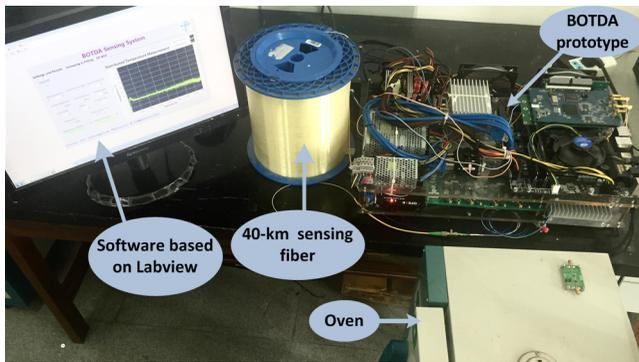
Fig. 3 BOTDA prototype based on the proposed scheme.
