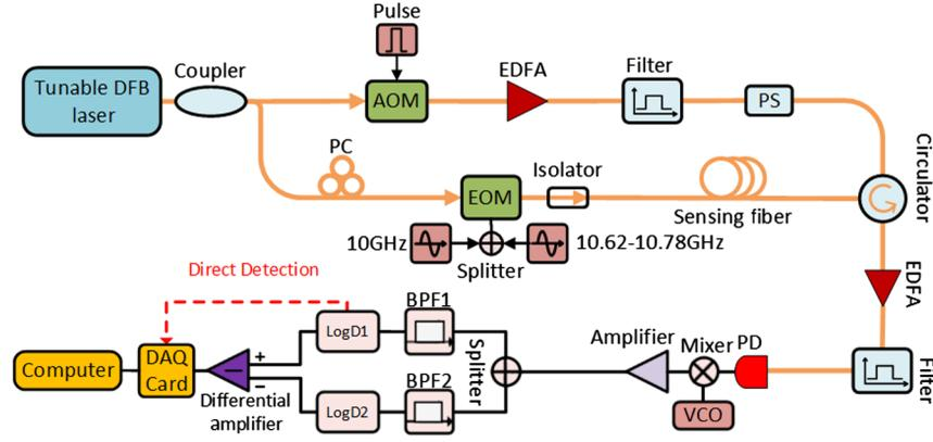
**Fig. 2** Experimental setup of the proposed coherent BOTDA sensor with DC component cancellation (path a), while path b shows the case without DC compensation. EDFA, erbium-doped fiber amplifier; PS, polarization scrambler; VCO, voltage-controlled oscillator; and BPF, bandpass filter.
