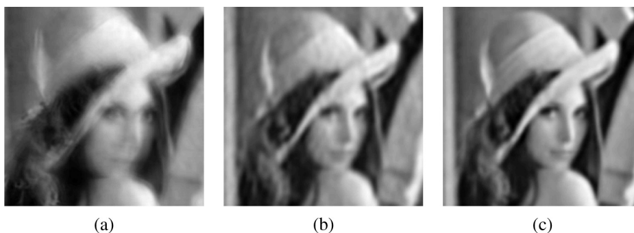
Fig. 22 Using speckle imaging (SI) to jump start MFBD. (a) Low turbulence condition input image sample, (b) initial estimate from SI as MFBD starting point, and (c) B-MFBD output when run to convergence.
