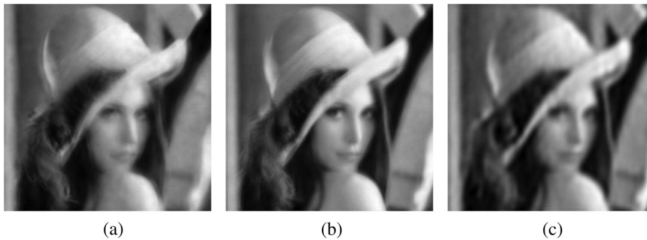
Fig. 3 Gaussian noise model Case 1 sample images. Compares (a) a sample turbulent image, (b) a sample MFBD-reconstructed object, and (c) a sample bispectrum-reconstructed object.
