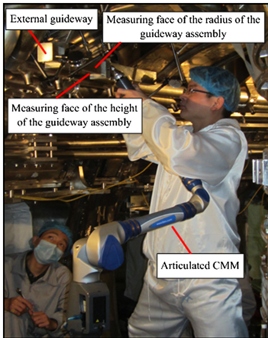
Fig. 7 External guideway assembly inspected by articulated CMM.
