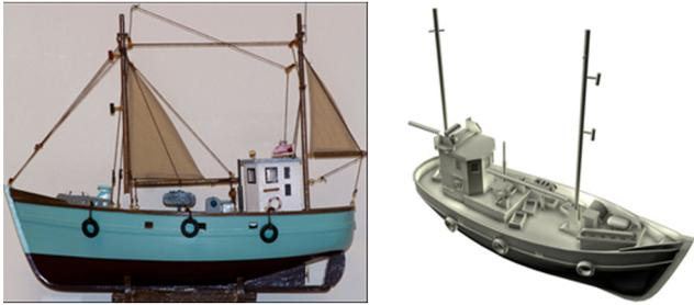
**Fig. 2** Toy model of a 43-cm long and 13-cm wide fishing boat. (a) A photo, and (b) a simplified three-dimensional (3-D) model (without sails and connecting ropes) used for simulating the waveform return from a laser profiling system. The model did not take into account any differences in reflectivity from the various parts of the boat.
