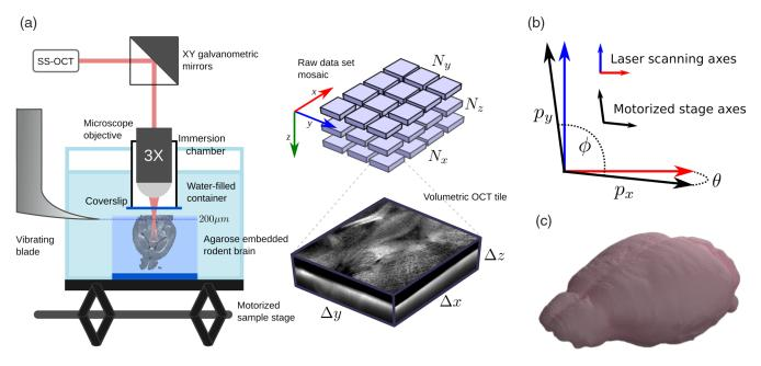
**Fig. 1** (a) Main components of the serial massive histology setup. (b) Parameters of the motor displacement model. (c) Volume rendering of a reconstructed brain (visualization made with the Blender software<sup>29</sup>).
