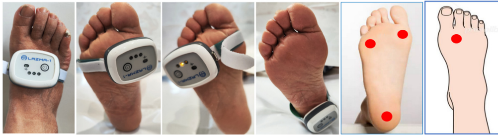
Fig. 1 Test equipment and parts below M1, below M5, heel, dorsum of the foot, and between the first and second metatarsals.
