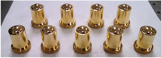
Fig. 14 Image of the cat's eye calibration test surfaces.
