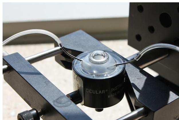
**Fig. 3** Photograph of the custom-built ocular model. Note that the chamber is fitted with two infusion tubes, which allows changing of glucose concentration in the anterior section.
