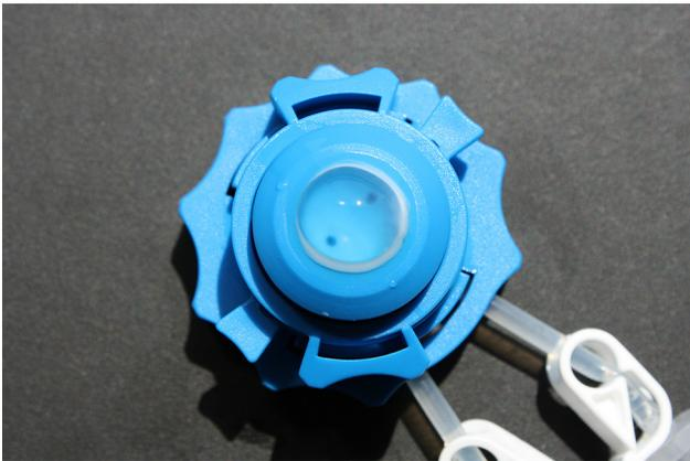
**Fig. 4** Photograph of an isolated cornea clamped on the artificial anterior chamber. Note that the clamping region is within the sclera, which can minimize stress on the cornea.
