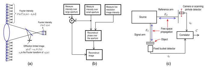
Fig. 34 (a) Principle of phase retrieval using a low-resolution image, (b) reconstruction of a fine-resolution image from the intensity measurements, and (c) ghost-imaging architecture.
