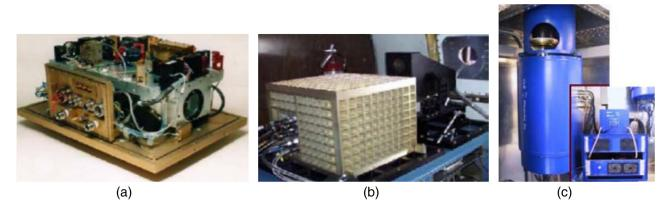
**Fig. 11** Wind sensors: (a) NASA optical air turbulence sensor (2  $\mu$ m, 1 mJ, 1 kHz, 5 cm aperture, chiller), (b) NASA ACLAIM turbulence warning (2  $\mu$ m, 8 to 10 mJ, 100 Hz, 10 cm aperture, chiller), and (c) MAG-1A WindTracer (2  $\mu$ m, 2 mJ, 500 Hz, 10 cm aperture, heat exchanger).
