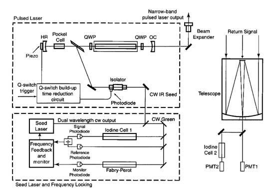
Fig. 7 Schematic diagram for injection-seeded Q-switched pulsed Nd:YAG laser transmitter.<sup>26</sup>
