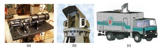
**Fig. 16** Lidars for atmosphere investigation: (a) all-fiber coherent multifunctional CW laser radar for range, speed, vibration, and wind measurements at 1.55  $\mu$ m (FOI, 2000), (b) Lidar automatic system for remote air pollution monitoring in large industrial areas (former Institute of Precision Instrumentation, Moscow), and (c) multifunctional lidar system (Astrofizika Corporation, Moscow).
