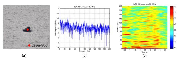
**Fig. 13** Vibration measurements from a rubber boat. (a) Visible image with marked laser beam, (b) frequency spectrum of the velocity, and (c) frequency spectrum over time.
