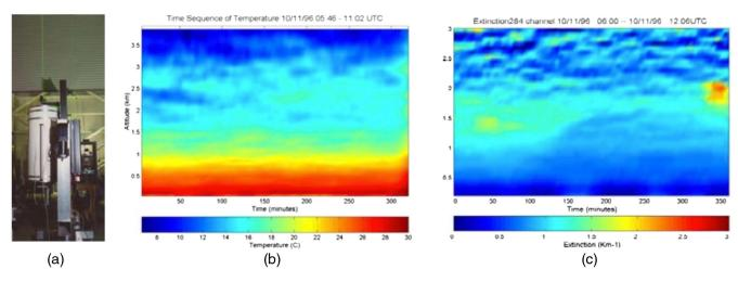
Fig. 17 (a) Lidar at the Pennsylvania State University and (b and c) dynamics of temperature and extinction.
