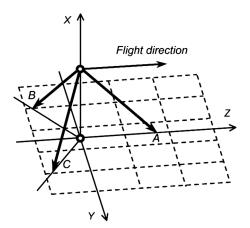
Fig. 10 Unit vectors describing the sensor geometry.
