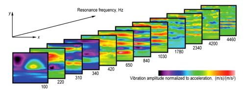
Fig. 15 Resonance vibration frequencies registered in the cabin of the helicopter mock-up.
