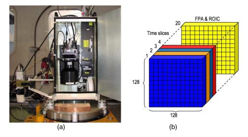
Fig. 25 Airborne flash laser radar developed by Northrop Grumman Aerospace Systems: (a) general view and (b) principle explanation.
