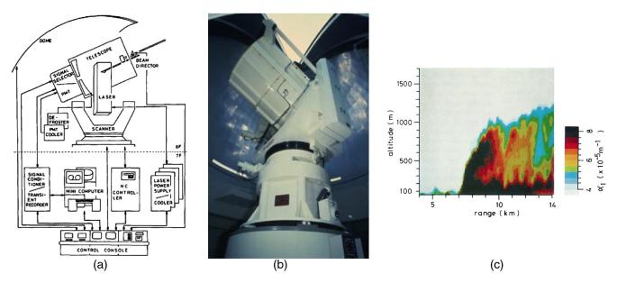
Fig. 20 Large scanning lidar system (NIES): (a) schematic diagram, (b) photo of the lidar, and (c) structure of sea breeze front.
