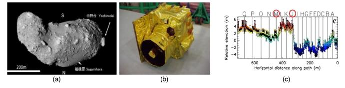
Fig. 4 "Hayabusa" mission using the Hayabusa lidar. (a) A picture of the asteroid "Itokawa" taken by an imager, (b) a flight model, and (c) relative elevation and horizontal distance measured by the Hayabusa lidar.
