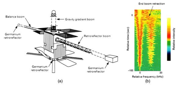
Fig. 14 (a) LACE satellite. Relative vibration was measured between the germanium retroreflector located on the satellite body and the retroreflector located on the retroreflector boom tip. (b) Doppler-time-intensity representation of data aligned to the peak return.
