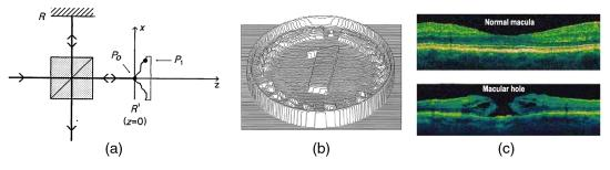
Fig. 30 (a) Basic setup of an optical microradar, (b) 3-D reconstruction of a coin image, and (c) eye bottom tomograms.
