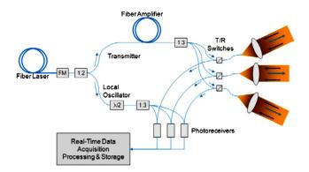
Fig. 9 Doppler lidar system configuration.
