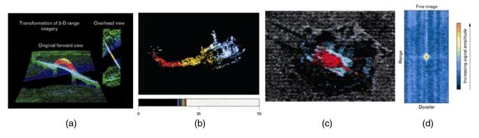
**Fig. 21** Images from MIT/LL laser radar systems: (a) CO<sub>2</sub> laser-radar images of a bridge, (b) Dopplervelocity image of a UH-1, (c) laser-radar image of a tank concealed by a camouflage net, and (d) range-Doppler image of the LAGEOS satellite collected by the wideband CO<sub>2</sub> laser radar at Firepond.
