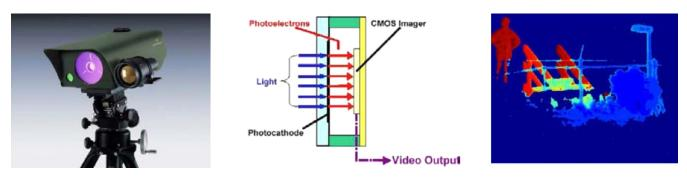
Fig. 26 Laser-gated viewing using Intevac Livar 4000 laser-gated viewer.
