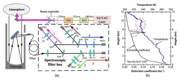
Fig. 18 (a) Vibration-rotational Raman lidar system developed at Xi'an University of Technology and (b) extinction and temperature profiles.
